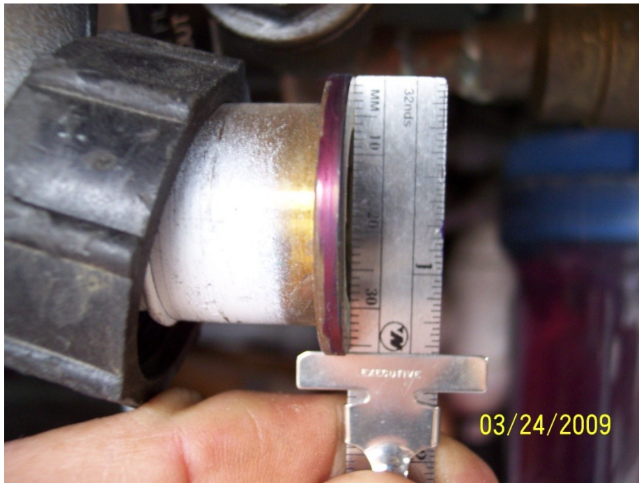
Bus Side Inlet & Outlet Line Diameters ( 36mm – 1 3/8" inch O.D. "Shoulder Diameter" ) ( 25mm – 1.00" inch I.D. " Opening Diameter " )
