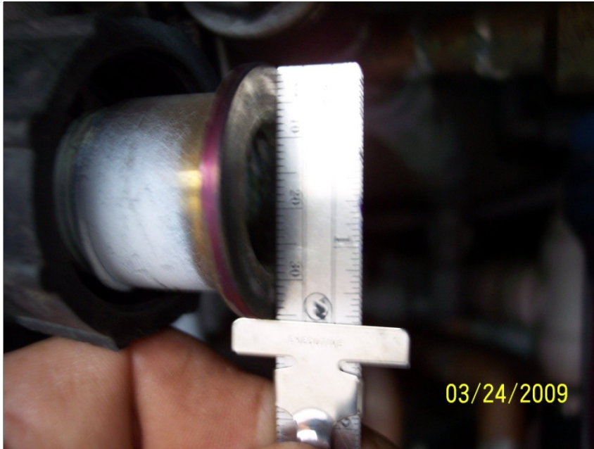
Bus Side Inlet & Outlet Line Diameters ( 36mm – 1 3/8" inch O.D. "Shoulder Diameter" ) ( 25mm – 1.00" inch I.D. " Opening Diameter " )
