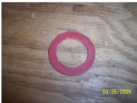
Final Cut of New Replacement Gasket
